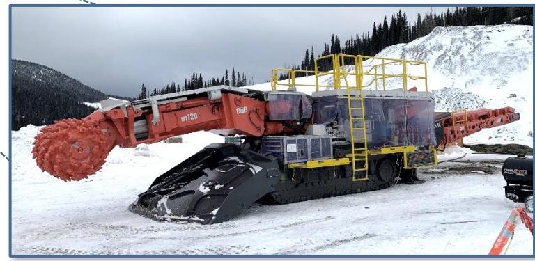
ROADHEADER AT SITE
